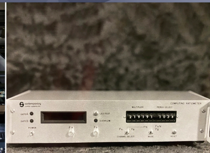
The first microprocessor-based computing ratiometer, developed by Contemporary Controls in 1975.
