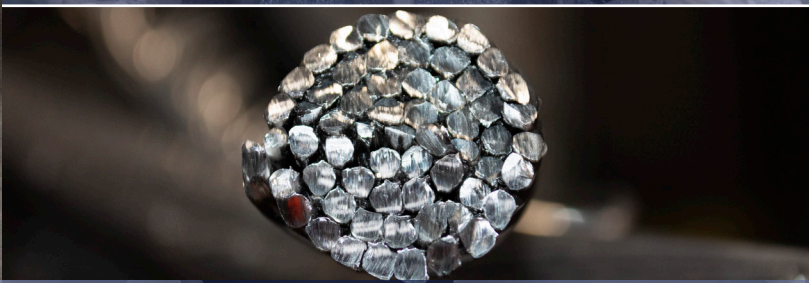
The cables come in many configurations. This cable is made of over 60 wires!
