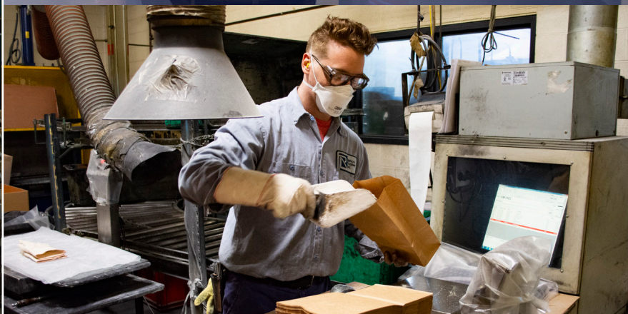
An employee measures chemicals by weight in order to make precisely-manufactured rubber compounds for different products.
