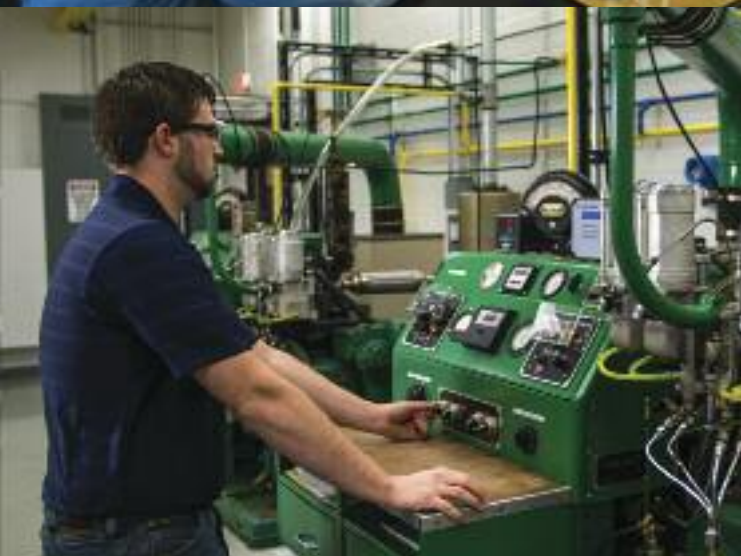
Falex's Lab Manager, (top photo) running a data analysis of a tribology test. A laboratory technician (bottom photo) running a fuel certification test for octane rating.
