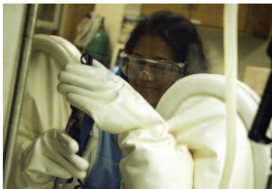
The use of isolators provides a controlled, sterile work environment that is less energy intensive than traditional manufacturing environments. Baxter has integrated the use of isolators into many of its facilities, including in Round Lake, Illinois.
