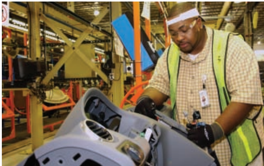
Ford Chicago Assembly Plant: An employee from Visteon Corporation, one of the suppliers manufacturing onsite at the Chicago Assembly Plant (CAP), is preparing to make electrical connections for audio and climate control systems.
