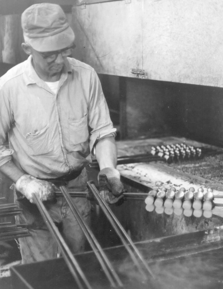
An employee quenches red-hot hammers in oil (1969).
